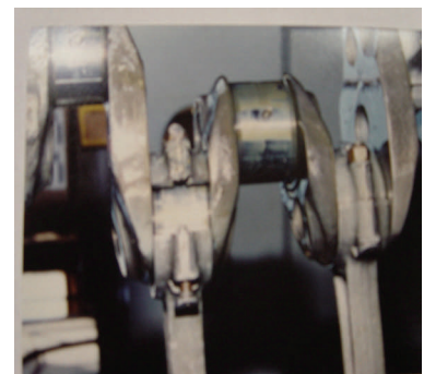
#4 Rod Missing, #3 Rod Bolt Broken
